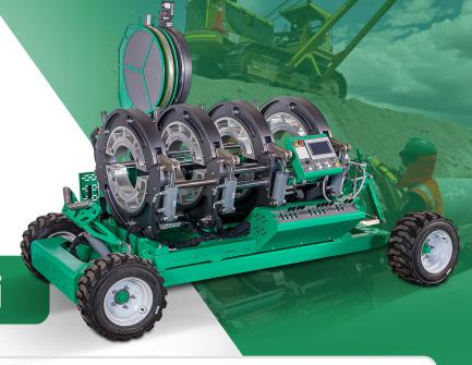
Riyang ARMOR 630i/24i is a high-performance fusion welding machine with trailer mobility, designed to excel on construction sites. It boasts a welding range from 200mm to 630mm or 8" to 24"IPS, adhering to ISO21307 and ASTM F2620 high-force standard. With a fully automated system featuring SIEMENS PLC technology, ARMOR 630i/24i ensures precision and reliability. Crafted from premium aluminum components, this machine guarantees strength and accuracy for all your welding needs.
